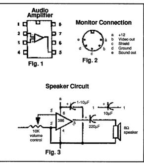
unfamiliar with how to read the pins on an integrated circuit, if you hold it in your hand with the pins facing down and you can read the marking on the chip, pin No. 1 is the one in the lower left corner.
