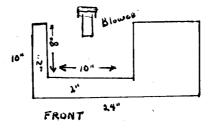
I used a 10-inch by 24-inch sheet of three-quarter inch plywood and cut out roughly an 8-inch by 10-inch piece from the left side and back, leaving about a 2inch border on the left side and front with an opening at the back. The console sits on this frame, and the cable and speech synthesizer rest on the right side.
