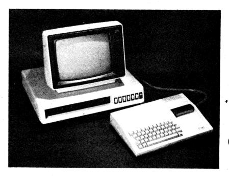
which has the CorComp 9900 system and TI speech synthesizer, built in along with the features of the TC-1. This configuration is a complete expansion system which will retail at about \$750.
