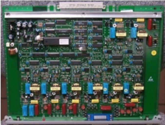
**Figure 2-8: LCOB-8 (8-Circuit Loop Start Board)**
