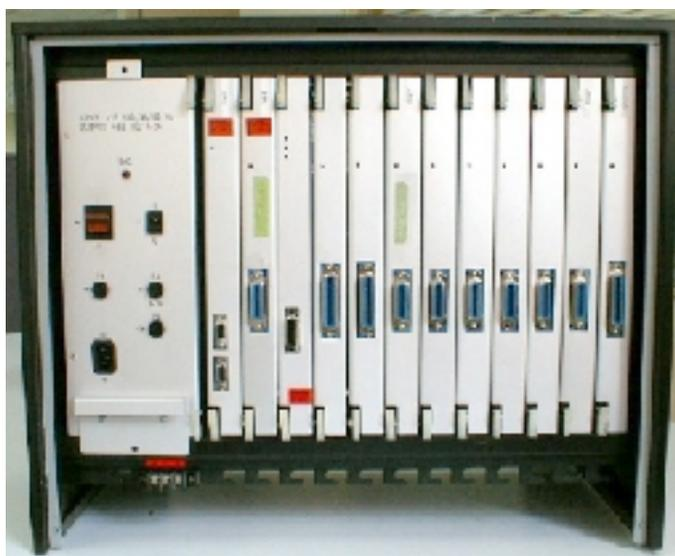
**Figure 2-1: DHS-L KSU (cover removed)**
