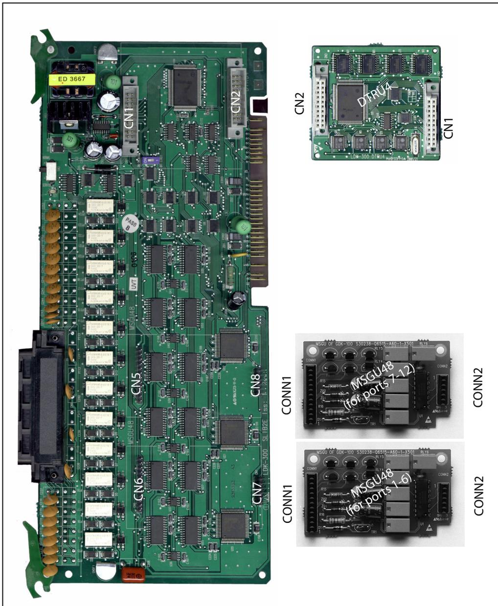
Figure 3-30: SLIBE & SLIBC w/MSGU and DTRU4 Module Installation
