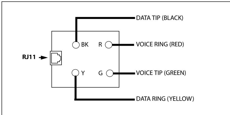
**Figure 3-38: Electronic Station Wiring**
