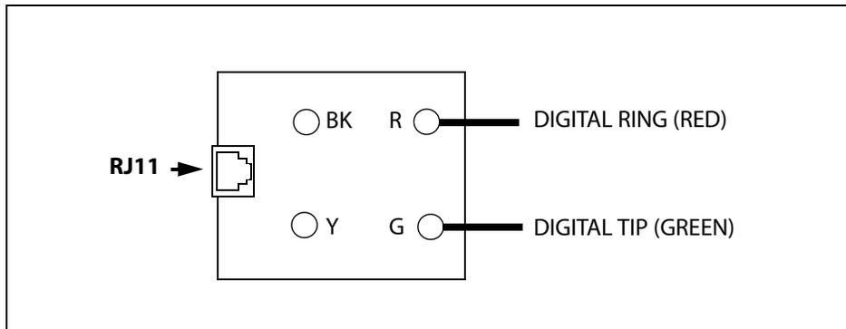
**Figure 3-37: Digital Station Jack Wiring**
