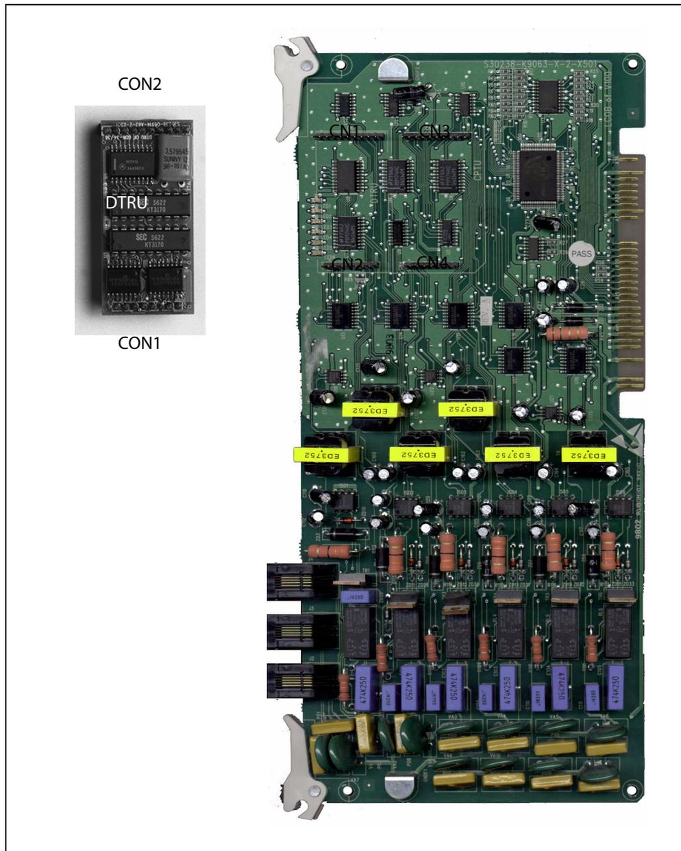
**Figure 3-15: LCOB Interface Board w/DTRU Installation**
