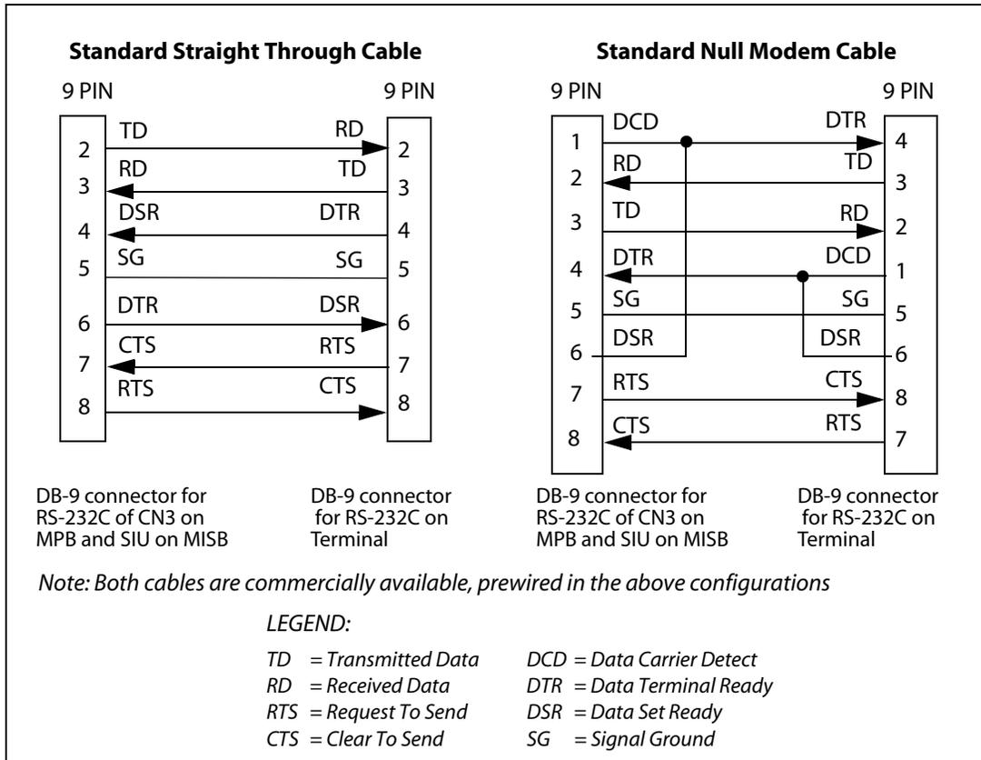
**Figure 3-33: RS-232 9-Pin Connector Cable Wiring**
