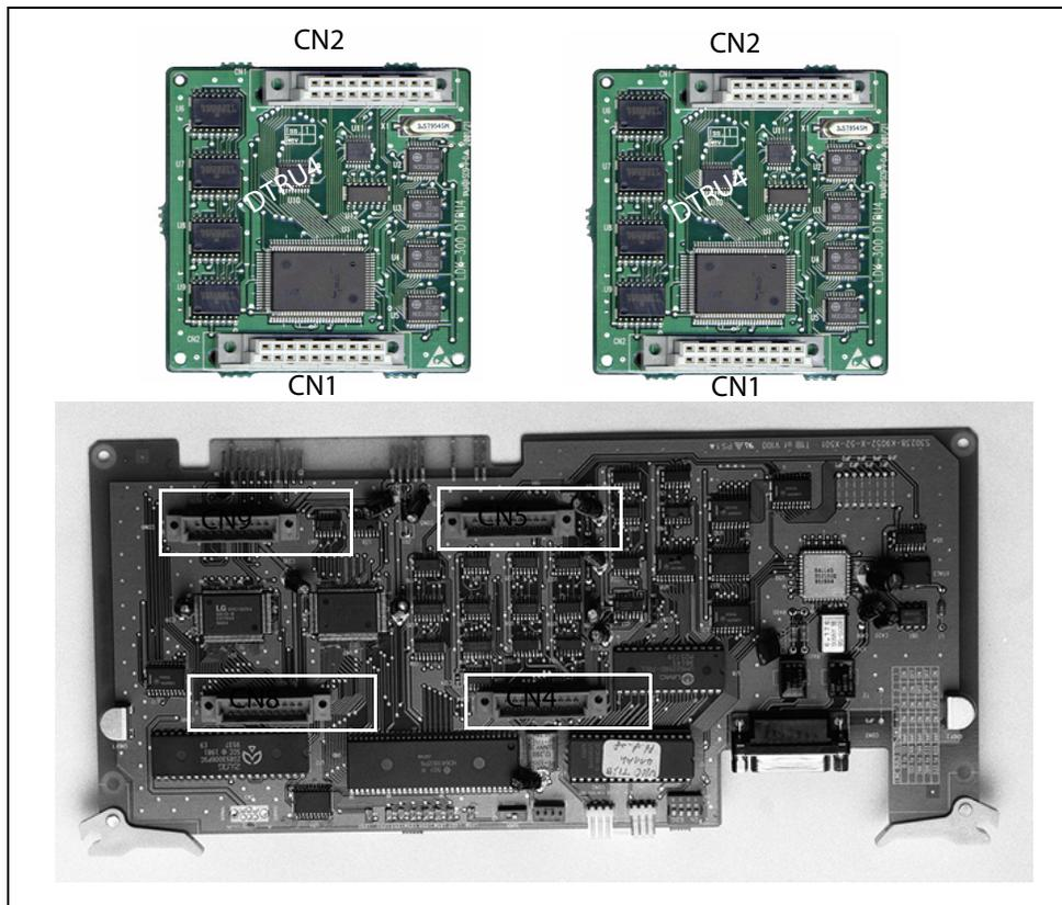
**Figure 3-18: T1IB w/DTRU4 Module Installation**
