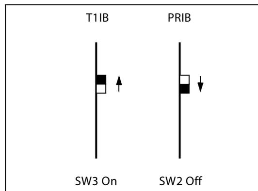
If both cards in a phone switch are connected to a telephone company clock (not point-to-point T1), put the T1 clock switch in the enable position (UP) to allow it to receive clocking from the telephone company directly, and do not install the clock cable.
