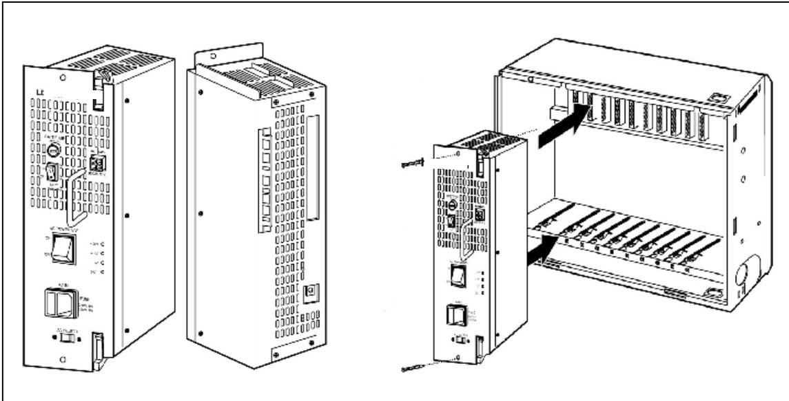
**Figure 3-8: PSU Installation**
