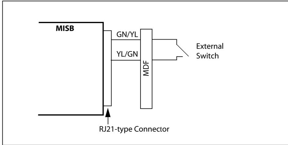
**Figure 3-36: External Switch / Alarm Wiring**
