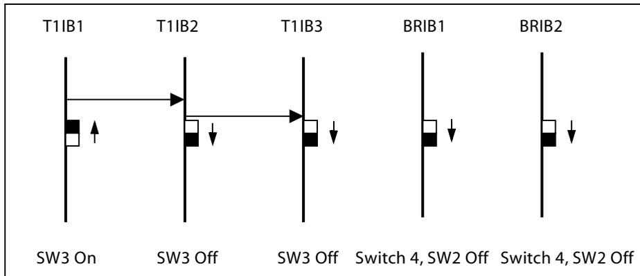
The clock OUT cable from T1IB1 should be connected to the clock IN cable of the T1IB2 and the clock OUT cable from T1IB2 should be connected to the clock IN cable of T1IB3. SW3 of T1IB1 should be in the ON position, and SW3 of T1IB2 and T1IB3 should be in the OFF position. The two BRIBs are not connected with clock control cables and SW2 of the BRIB cards are placed in the OFF position.
