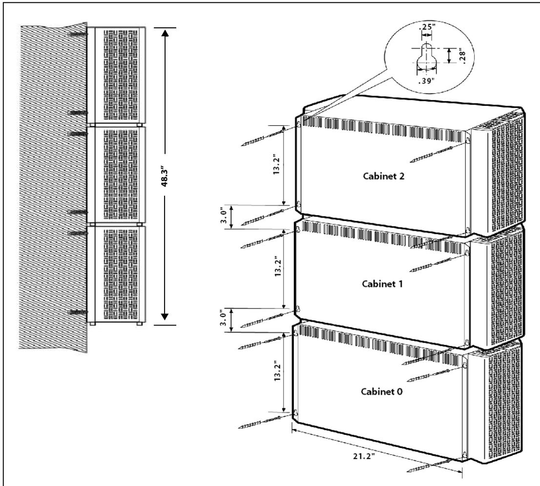
Figure 3-4: Mounting Cabinets 0, 1, & 2
