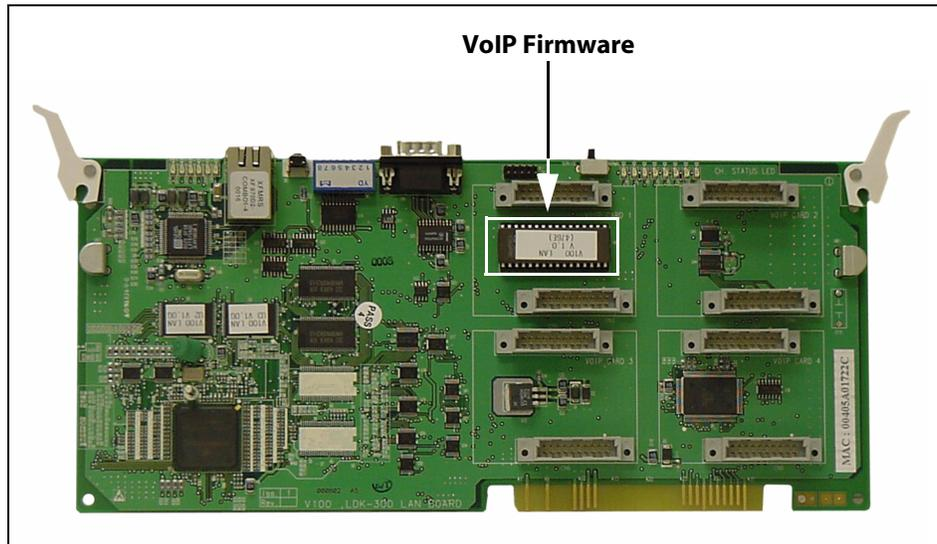
**Figure 3-22: VoIP Card - No VoIP Modules Installed**
