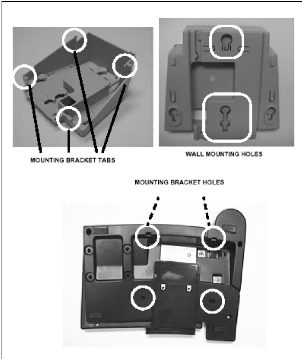
**Figure 3-42: Digital Key Telephone Wall Mounting**
