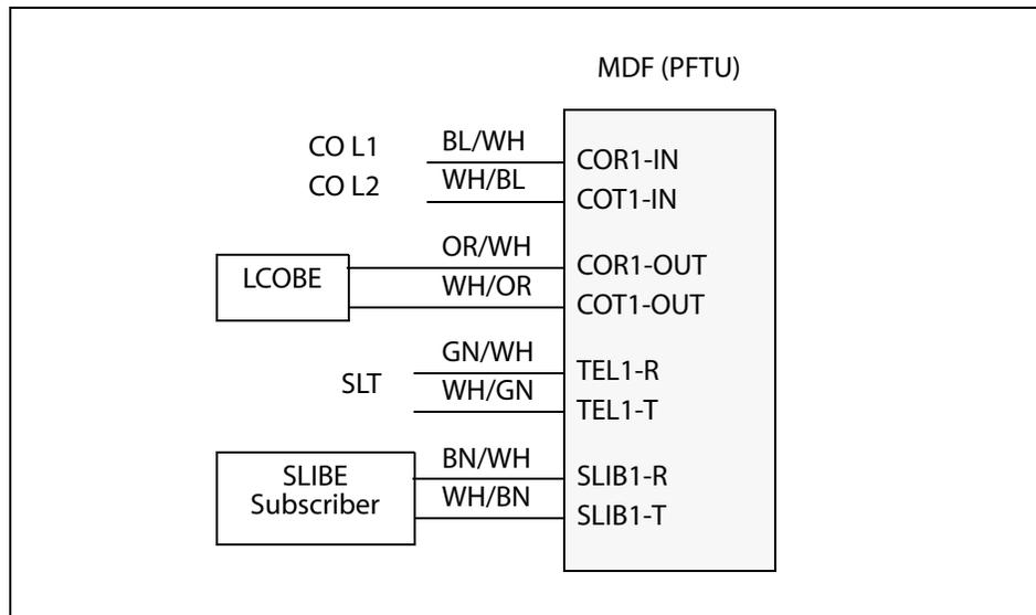
**Figure 3-40: PFTU Wiring**
