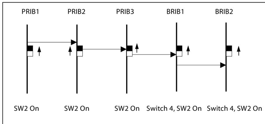
The clock cable should be connected from the OUT position of the PRIB1 to the IN connectors of all the cards and all clock switches should be in the ON position.
