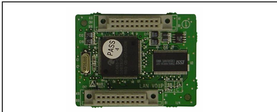
**Figure 3-23: Connection Side of VoIP Module (Closeup)**
