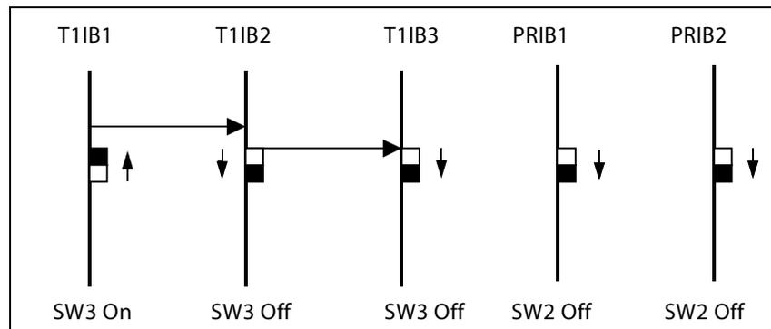
The clock cable should be connected to the OUT position on the cable connector on the T1IB1 and connected to the IN position on the connector on the T1IB2.
