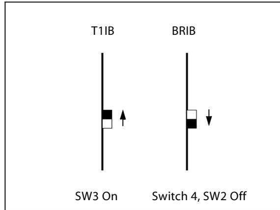
If both cards in a phone switch are connected to a telephone company clock (not point-to-point T1), put the T1 clock switch in the enable position (ON) to allow it to receive clocking from the telephone company directly. Do not install the clock cable.
