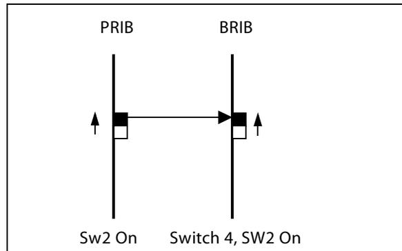
Install with the cable and set both PRIB and BRIB switches to the enable position (ON).
