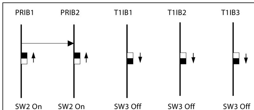
The clock cable should be connected to the OUT position on the connector on the PRIB1. The clock cable should be connected to the IN position on PRIB2. SW2 of the PRIB1 and PRIB2 should be placed in the ON position. The three T1IBs are not connected with the clock control cable and SW3 on these boards should be in the OFF position.
