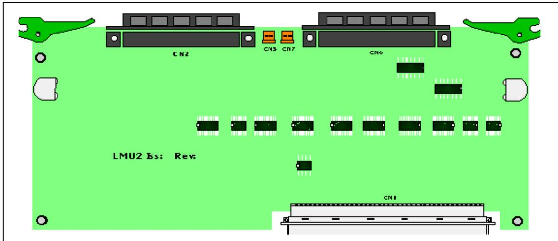
**Figure 3-12: LMU2 Board Configuration**
