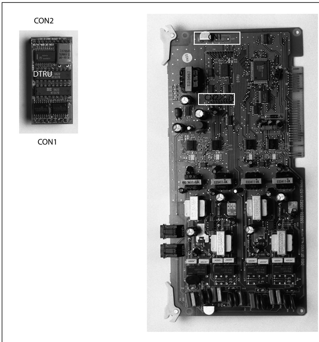
**Figure 3-17: DIDB w/DTRU Installation**
