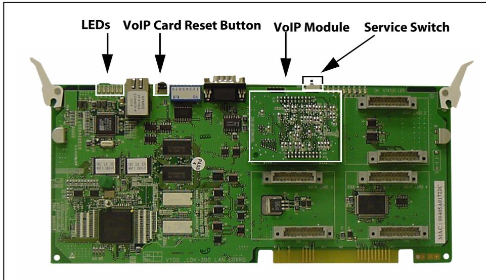
**Figure 3-21: VoIP Card with One VoIP Module Installed**
