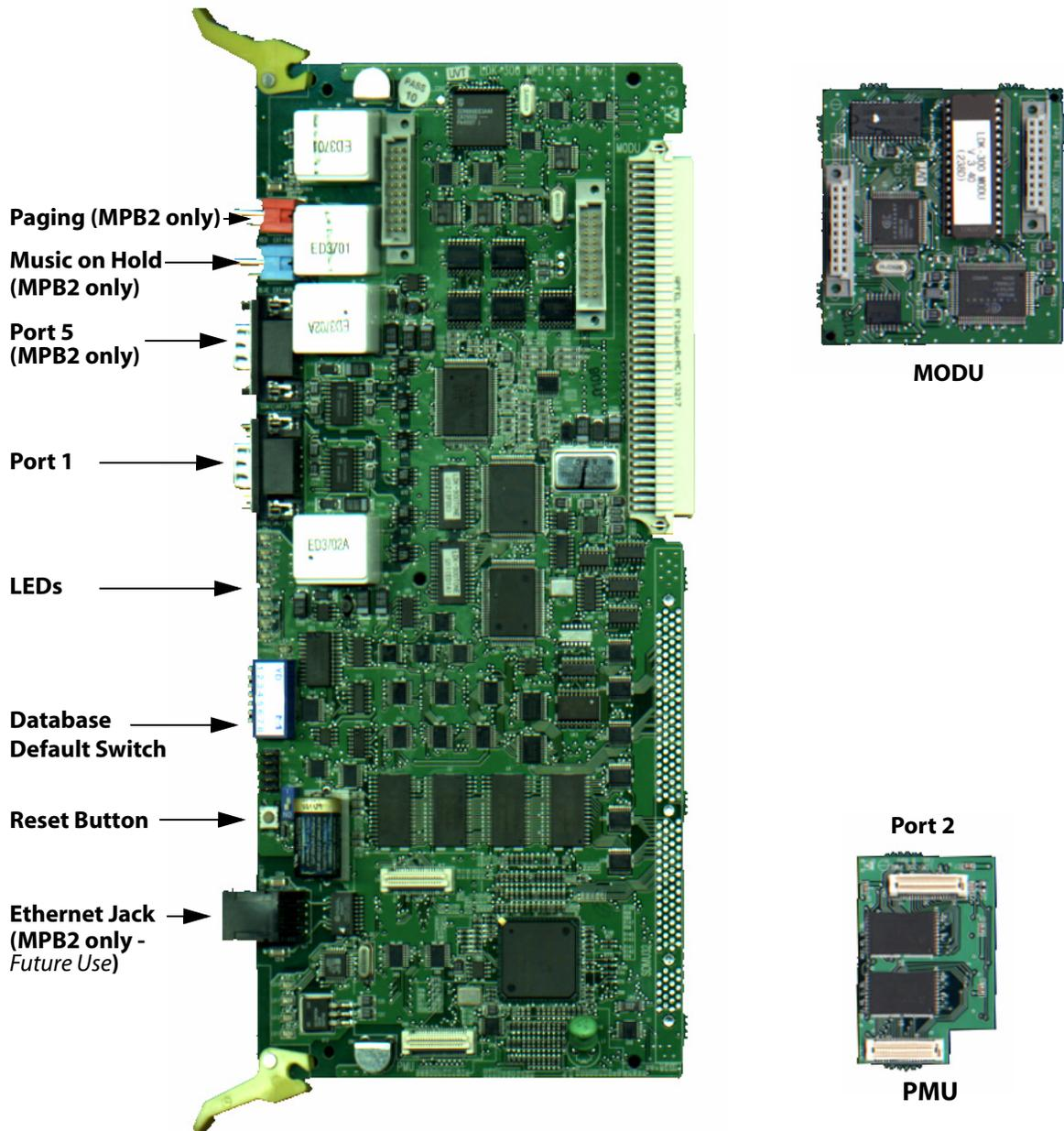
Figure 3-10: MPB, PMU, and MODU Configuration
