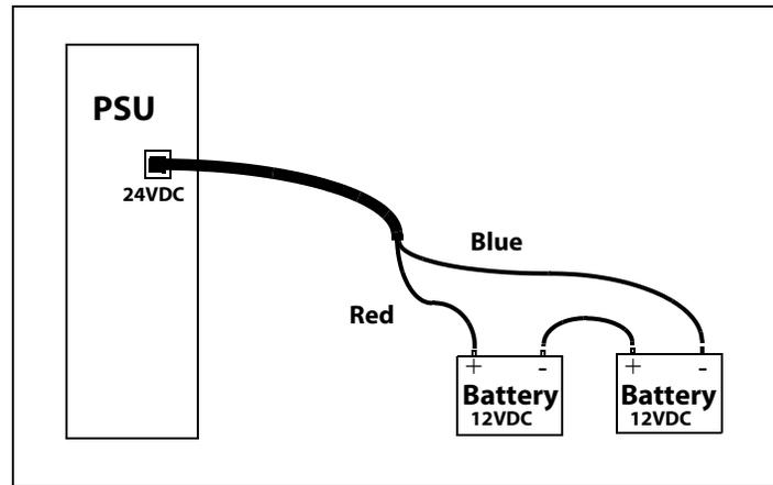
**Figure 3-32: Battery Back-Up Wiring**
