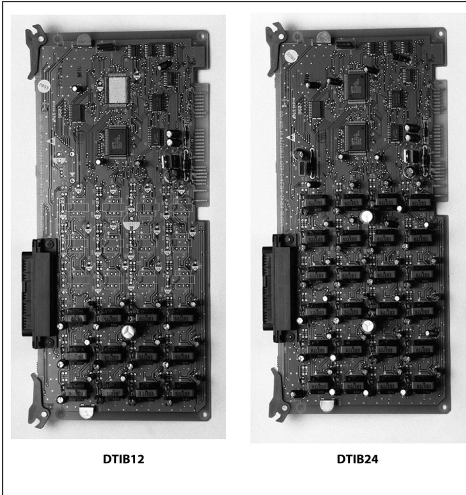
**Figure 3-31: Digital Telephone Interface Board (DTIB)**
