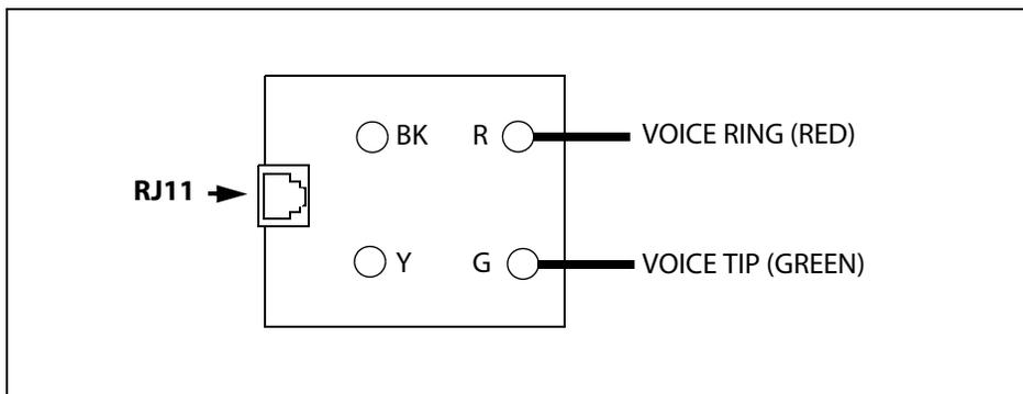
**Figure 3-39: Single Line Telephone Wiring**
