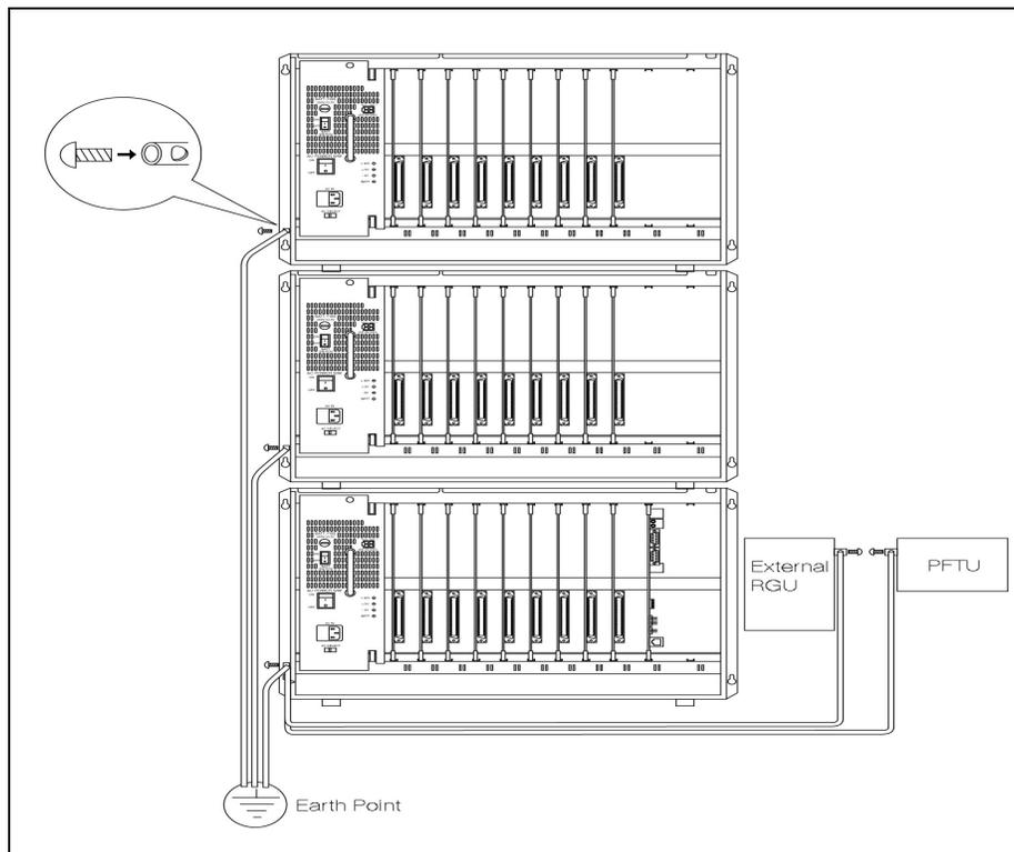
**Figure 3-5: Earth Cable between KSU and External RGU**
