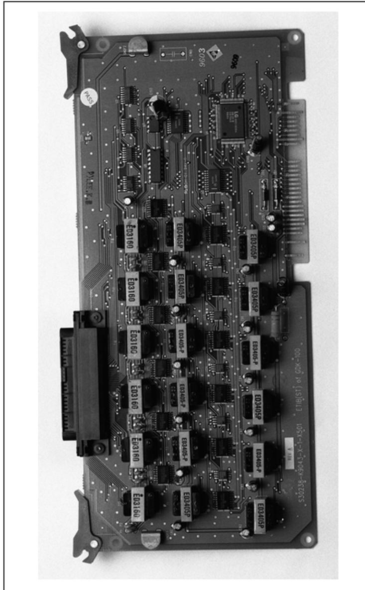
Figure 3-28: Electronic Telephone Interface Board (ETIB)
