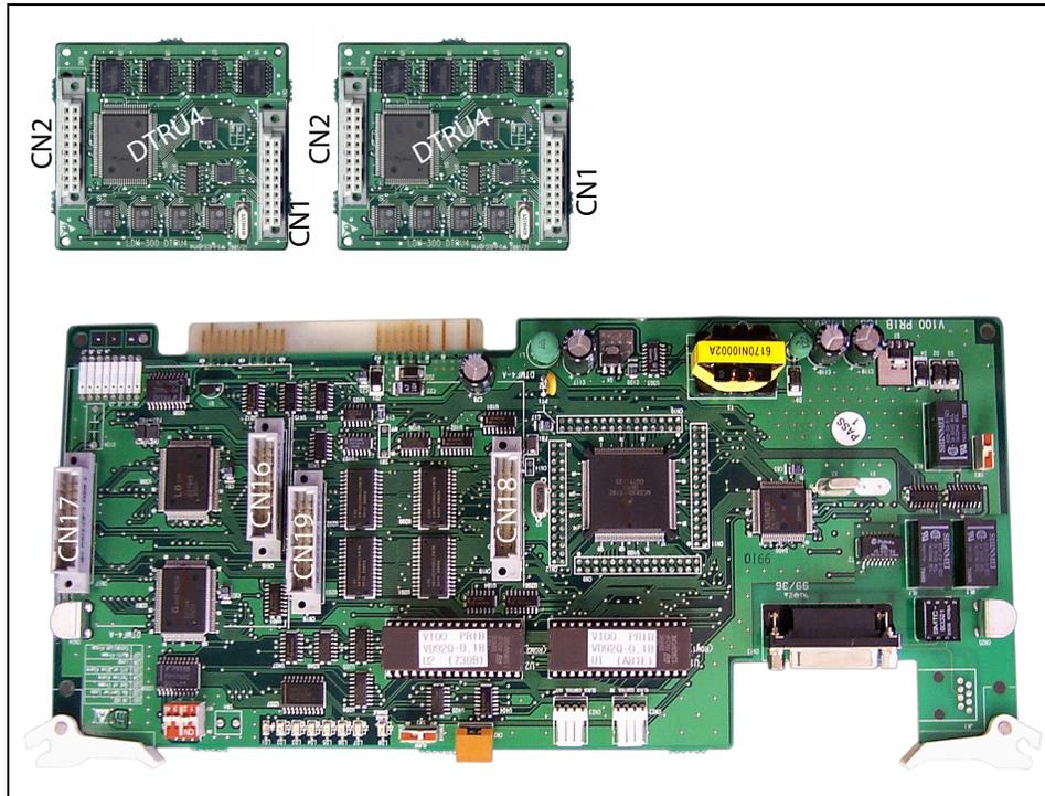
**Figure 3-19: PRIB w/DTRU4 Module Installation**
