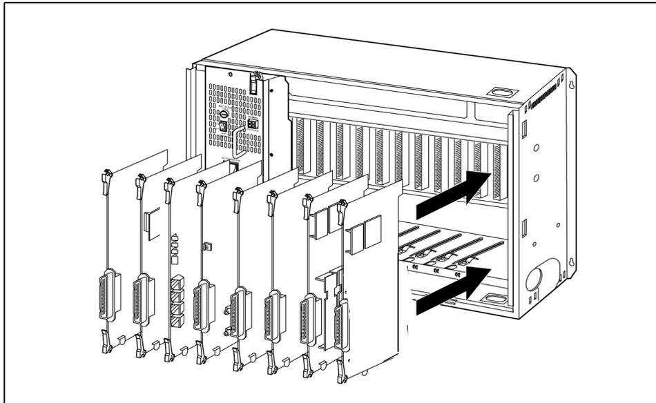
**Figure 3-9: PCB Installation**
