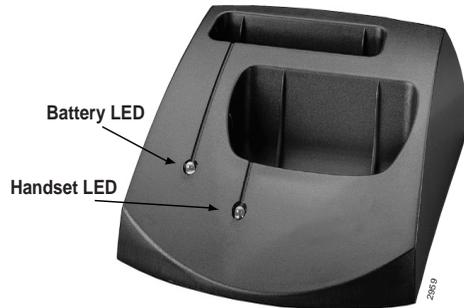
4. If you have a spare battery, insert it in the rear slot of the charger base.
