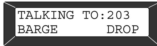
This display can be seen when investigating an intercom call. The investigator can BARGE-in or DROP the connection.
