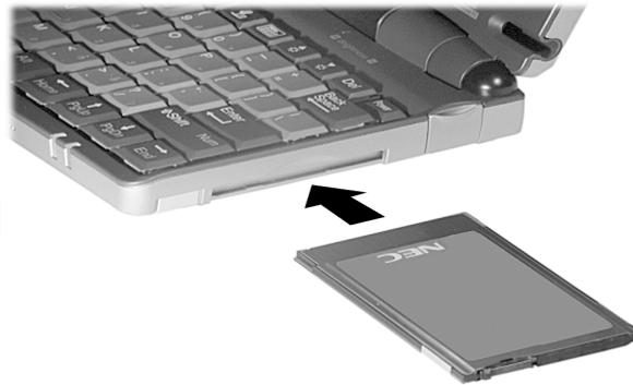
2. Verify that the PC card is fitted securely into position.
