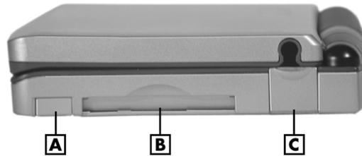
**A** – PC card eject button   **B** – PC card slot   **C** – Modem port
