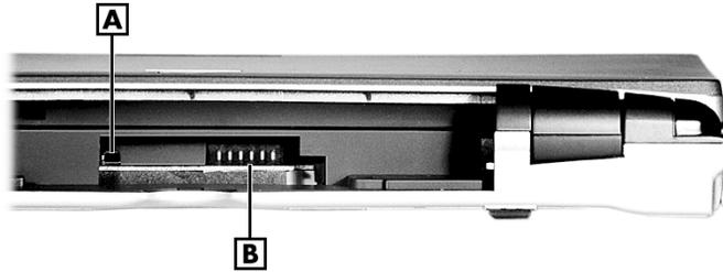
**A** – Full reset button **B** – Battery connectors
