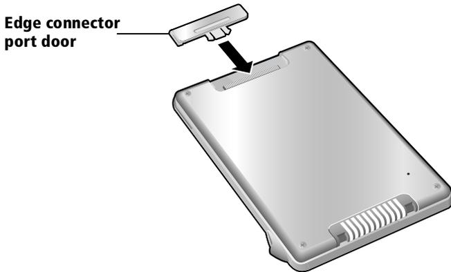
2. Insert the tab on the top edge of the edge connector port door into the edge connector port.
