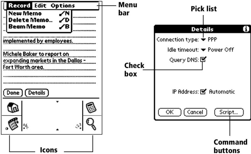
**Menu bar** A set of commands that are specific to the application. Not all applications have a menu bar.
