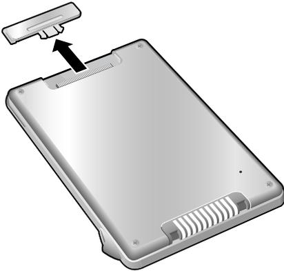
2. Slide the detachable Springboard slot onto the back of your handheld.
