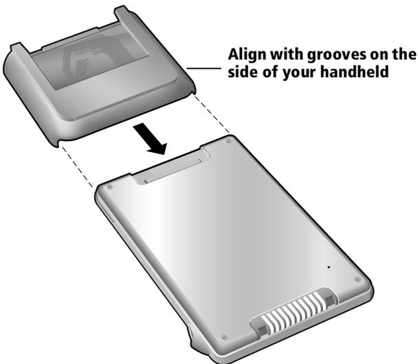
3. Insert the Springboard module into the expansion slot until the connectors are secure.
