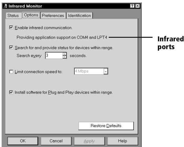
The COM port displayed on this screen is the port associated with your infrared device. It should be different from the port currently defined for cradle synchronization.
