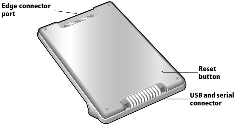
**Edge connector port** Enables you to connect the detachable Springboard slot. To install the detachable Springboard slot and add expansion modules to your handheld, you must first remove the flip cover or the edge connector door.
