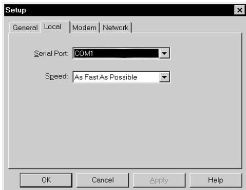
**Serial Port** Identifies the port that Palm Desktop software uses to communicate with the optional serial cradle. This selection should match the number of the port to which you connected the optional cradle.
