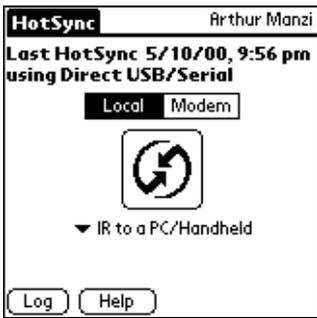
5. Position your handheld's IR port within a couple of inches of your computer's infrared port.
