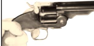
With your fingers outside of the trigger guard and a firm hold on the grips, place the thumb of your non-shooting hand on the hammer spur. Draw the hammer fully rearward until it is cocked as shown in (Figure 16). The revolver will now fire when the trigger is pulled.
