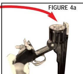
Push back the barrel latch and rotate the barrel downward. With the barrel pointed in a safe direction, continue to open the frame and barrel until the extractor completes its cycle and snaps back into the cylinder. (Figures 4 & 4a)
