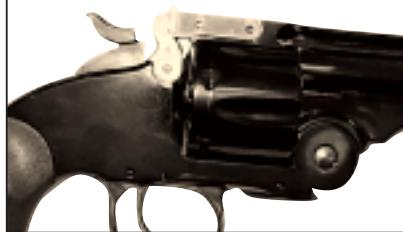
**NEVER ATTEMPT TO OPEN OR CLOSE THE BARREL/FRAME WITH THE HAMMER IN THE "AT REST" POSITION. FAILURE TO FOLLOW THIS WARNING WILL CAUSE DAMAGE TO YOUR FIREARM.**
