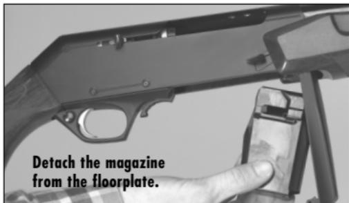
floorplate into place until retained by the magazine latch. If a round has already been placed into the chamber with the action open, a round may be chambered by depressing the bolt release lever and allowing the bolt to slam closed. If the action is closed, a round may be loaded into the chamber by pulling the operating handle rearward and releasing it.
