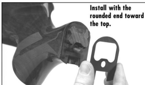
to scratch or mar the buttstock, and remove the recoil pad (Figure 10). Using a long shaft flathead screwdriver, loosen the stock bolt completely by turning in a counterclockwise direction, and remove the stock bolt (Figure 11). Completely remove the buttstock from the receiver. At this point you may add or remove the desired number of spacers. When adding spacers, make sure the rounded end of the spacers is installed towards the top of the rifle (Figure 12). When finished, fit the
