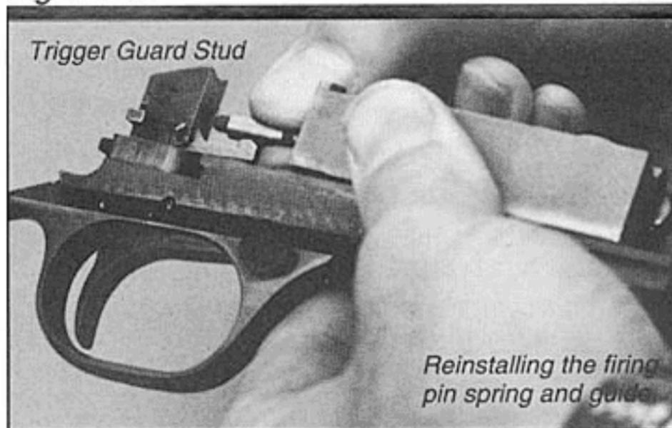
of the guide in the recess found in the trigger guard stud (see Figure 18).
