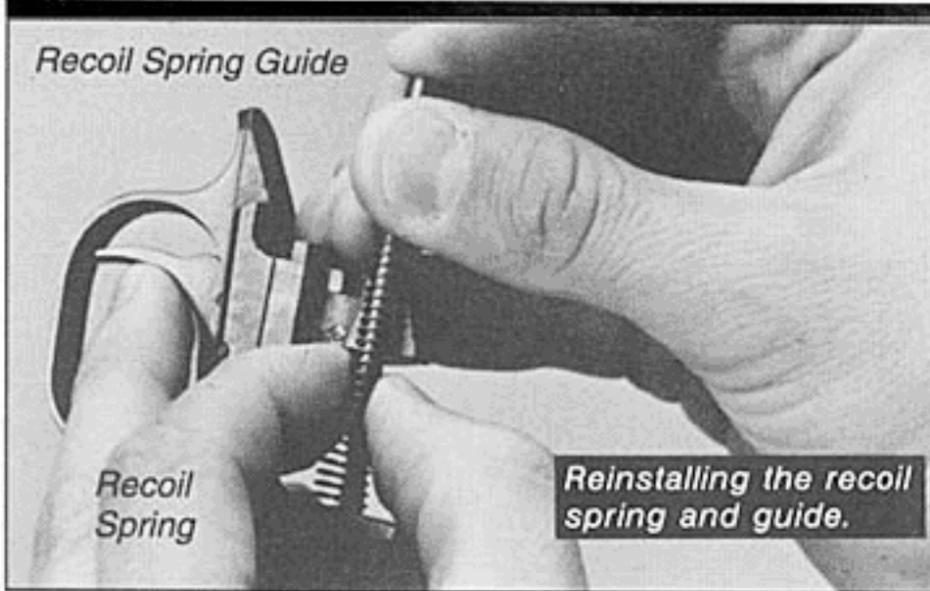
guide inserted in the other end, into the recoil spring hole of the breechblock.
