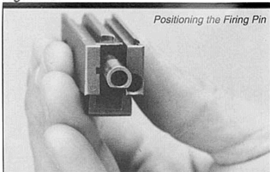
firing pin is inserted pin end first. Line up the firing pin so that the pin portion of the firing pin aligns with the firing pin hole located at the front of the breechblock — the flattened edge on the rear of the firing pin will be facing downward (see Figure 16).
