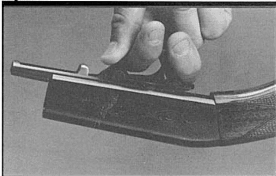
ejection opening to make sure no cartridge is left in the chamber. Then, check visually by holding the breechblock rearward with the thumb and looking into the receiver cavity, paying special attention to the magazine feed mechanism, to be sure no cartridges remain.
