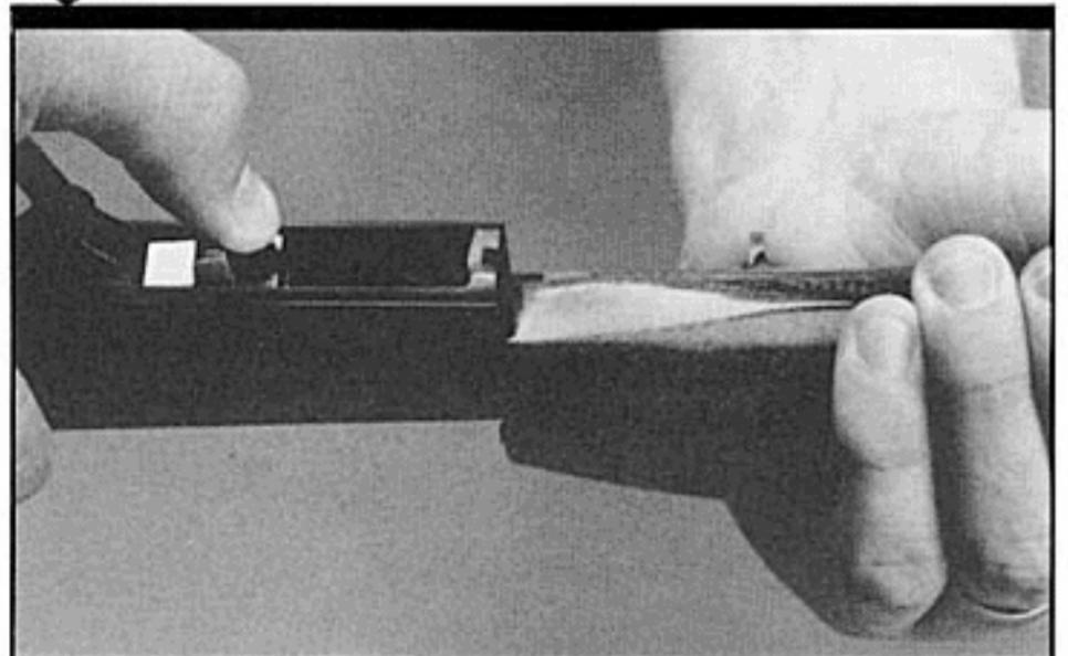
breechblock to go fully forward. Lock the barrel into position by drawing the barrel lock rearward (see Figure 4).
