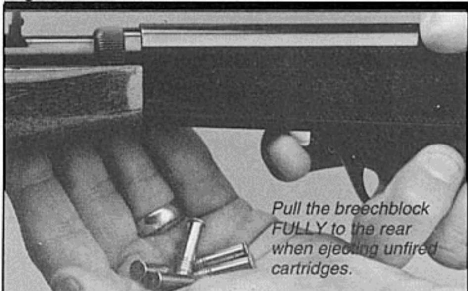
*Pull the breechblock FULLY to the rear when ejecting unfired cartridges.*
