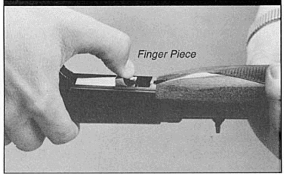
about 1/2" with your thumb (see Figure 3). Insert the barrel into the *receiver* as far as it will go. Be sure to hold the receiver when turning the barrel to connect it to the receiver. **HOLDING THE GUN BY THE STOCK DURING THIS PROCEDURE MAY DAMAGE THE STOCK.** Turn the receiver clockwise 1/4 turn until it stops in proper alignment with the receiver/stock: sights on top and forearm down. Release the finger piece allowing the
