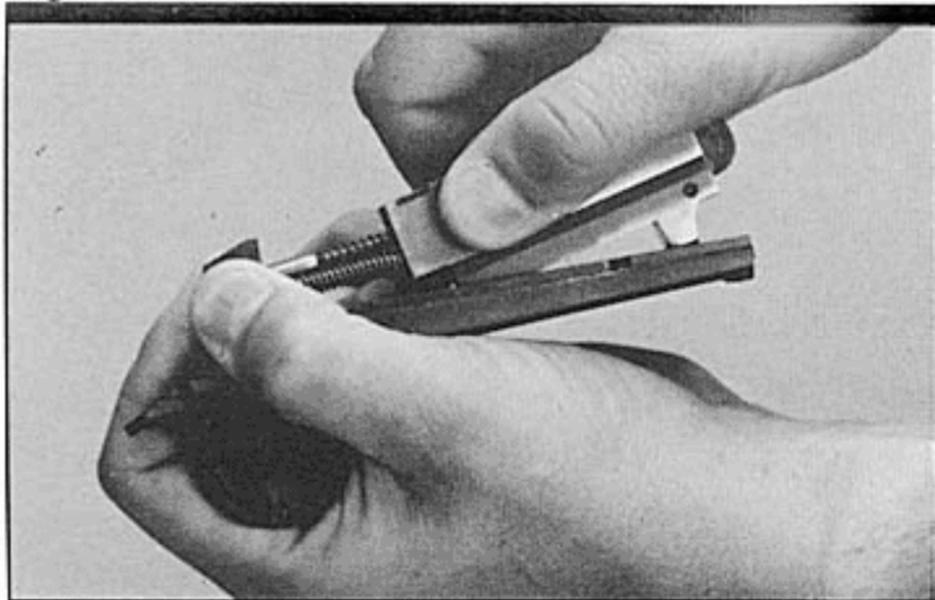
by pulling the trigger. Draw the breechblock back 1/4", then lift up on the forward end until the finger piece clears the trigger guard plate (see Figure 13). Allow the breechblock to travel forward slowly, holding the recoil spring between thumb and fingers to prevent its escape.
