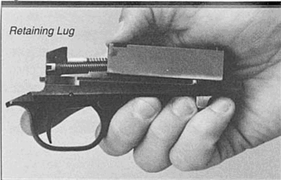
til the end of the recoil spring guide can be released against its retaining lug on the trigger guard stud (see Figure 20).
