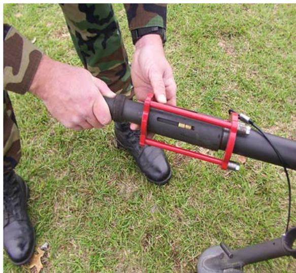
***F. In cool weather, water from propellant gasses may condense on the insert or Mk19 barrel. Wipe them clean and dry, then oil them to prevent damage to either.***
