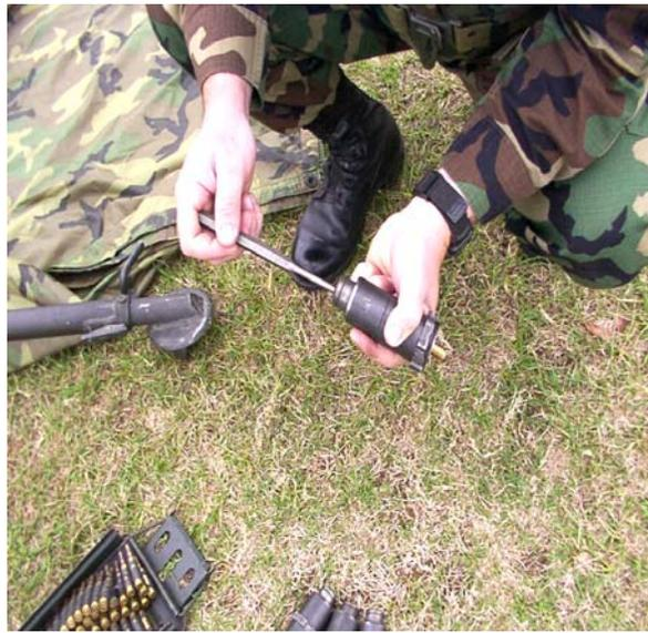
B. Insert each adapter cartridge base-down in the opening of the link positioning tube. Push the adapter cartridge into the link positioning tube to push the cartridge links forward until they stop.
