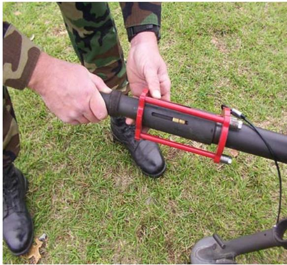
D. Pinch the front retainers of the Mk19's feed chute and swing the front outward. Insert the round discriminator (the red piece attached to the yoke with a cable) into the mounting point for the front retainers of the feed chute. The cable may be wound around the barrel to remove slack.
