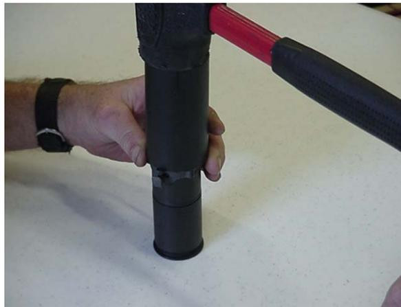
D. Use the link positioning tool to press the new link back until it passes the groove at the middle of the adapter cartridge, then use the tool to push it back into the groove.
