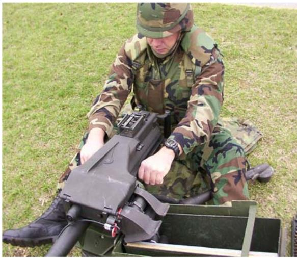
3. Push the chargers forward and rotate the charger handles up to the operational position.
