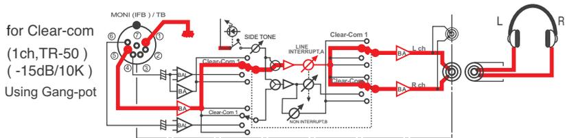
This signal is at -15 dB and with an impedance of 10 kΩ.
