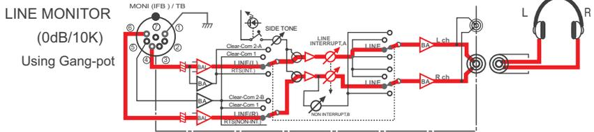
These signals are at 0 dB and with an impedance of 10 kΩ.
