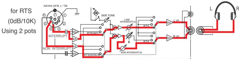
These signals are at 0 dB and with an impedance of 10 kΩ.
