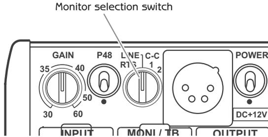
Note that depending on the switch setting here, the wiring assignment of the **MONI/TR** 7-pin XLR connector on the rear panel will change. See the specifications for full details.
