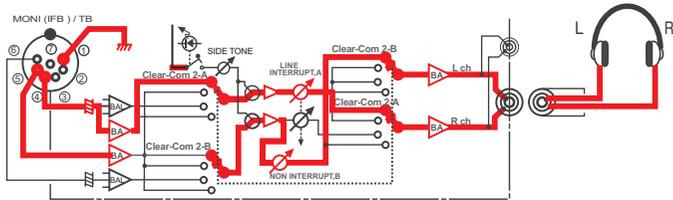
These signals are at -15 dB and with an impedance of 10 kΩ.
