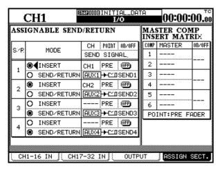
Assignable send/returns 1 and 2 should be set to the insert mode.
