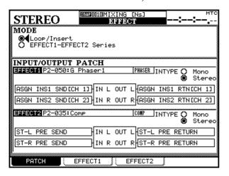
The stereo compressor assigned to effect 2 is inserted in the stereo output buss in order to limit the dynamic range of the stereo outputs.
