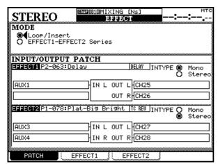
Press the **EFFECT** key followed by soft key 1 (PATCH) to bring up the patch screen as shown here.
