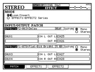
The stereo inputs to the plate reverb maintain the image of the stereo source (for example, if a pair of overhead mics has been set up to record a drum kit).
