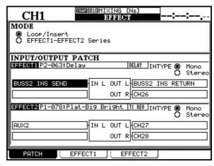
Select BUSS2 INS SEND as the input source for effect 1. When you do this, the output for effect 1 will automatically change (BUSS INS RETURN).
