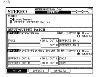
These echoes are then passed to the reverb, where they are processed "in-place" to provide an interesting stereo effect (note that reversing these two effects would produce echoed reverb—probably less desirable).
