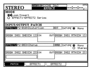
Effect 2 (a chorus) is inserted into an input channel (for example, a fretless bass) in order to thicken the sound. In this example, because these effects are being used by only one channel each, there is no need to tie up the aux sends and returns, which can then be used for other purposes.
