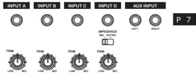
Inputs on the 788 can be routed directly to a mixer channel, or they can be assigned to the submixer. On the main mixer, any input can be assigned to any channel.
