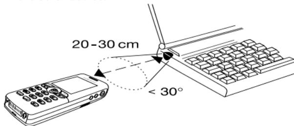
**Note:** If you are connecting to a PC, make sure your PC has activated infrared communication (*Start, Settings, Control Panel, Infrared, Options tab, Enable infrared communication*).
