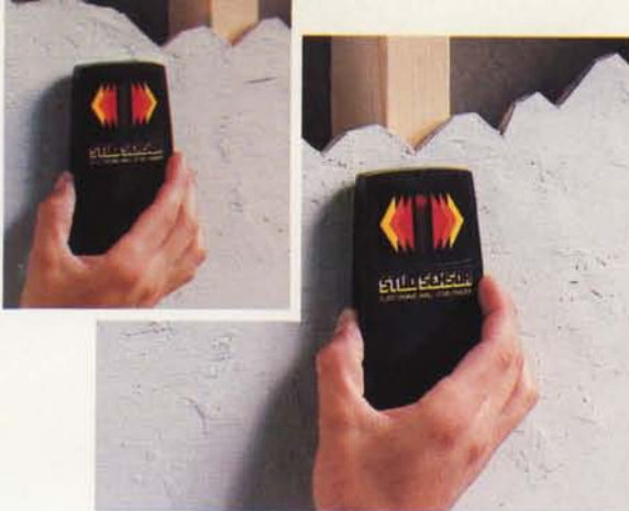
Stud Sensor "senses" density of wallboard. LED light signals change in mass as it passes over left edge of stud or joist. Once past stud, LED goes off indicating width of stud.
