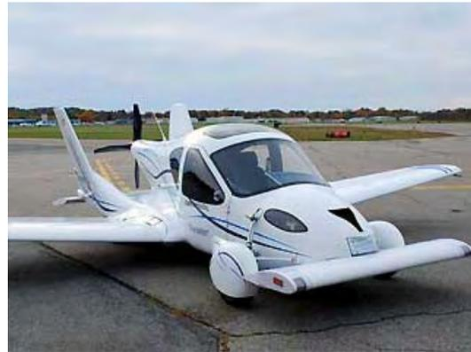
Called the Terrafugia *Transition* it can transform from a two-seater car to a plane in 15 seconds. The manufacturer claims it's easy to keep and run since it uses normal unleaded fuel and fits into a garage. The head of Terrafugia, said: "This is the first really integrated design where the wings fold up automatically and all the parts are in one vehicle."
