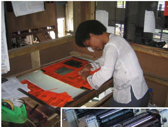
Stencils are cut for each colour and burned to light-sensitive aluminium plates.
