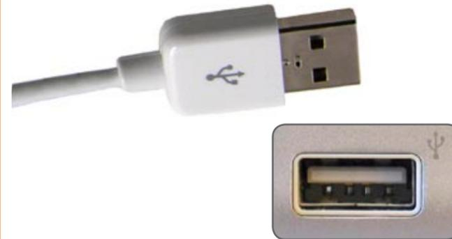
From 2001 to mid-2003, if you wanted to use an iPod, you needed to have a computer with **FireWire** - a high-speed data port developed by Apple. But today's iPods have dropped FireWire for the ubiquitous **USB 2.0** standard, a rectangular hole (shown at left) found on every computer shipped for the past year or two. Just like FireWire, USB 2.0 provides both power for your iPod and the ability to transfer data back and forth between connected devices.
